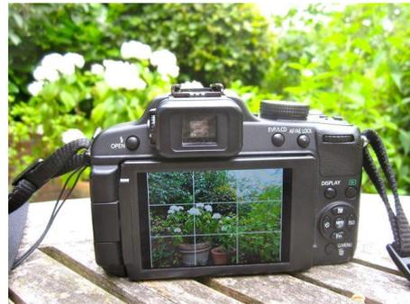
Figure 1 and 2: a digital camera with 24X optical zoom and 14 megapixels (source: KHLim)
